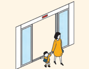
Safety feature works (opening or stopping the door) to prevent an accident.
